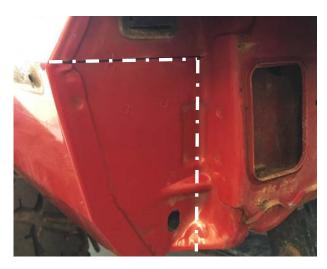
D.) Mark the cut line located on the front side of the rear corner and the inner fender well using a similar process as in the previous step. Masking tape can be used to match the contour of the metal to ensure a straight cut line is made. (**Note:** Find where the inner fender and the floor meet prior to marking your cut line to ensure you do not cut through the floor. This area should be about 1/4" above the bottom edge of the inner fender.)
