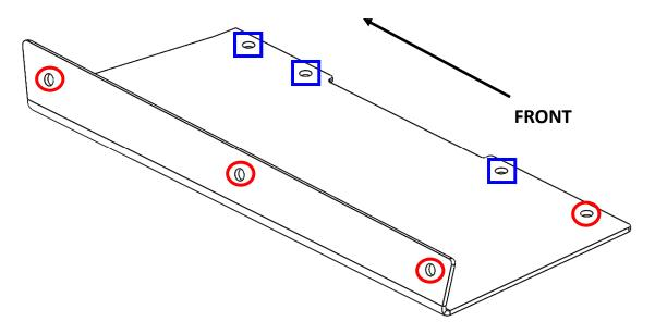
Drill hole to 3/8" then install 1/4" thread insert and fasten with 1/4" x 3/4 SS button head cap screw.
