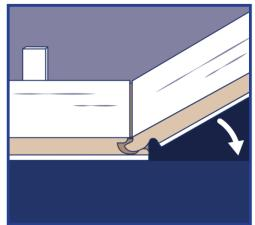
Step 2: Lock short end of flooring by inserting tongue into groove at an angle and drop in place. At end of the row, measure and cut the flooring to complete the row. Install the cut edge closest to the wall.
