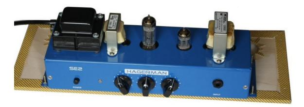
Insert power cord. Add supplied cable clamp to secure power cord to back panel, insuring strain relief. Install tubes (EL84 in larger hole) and mount assembly onto back of cabinet. Plug in speaker. You are ready to go!
