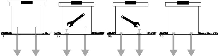
\*\*After install if the Boxx is difficult to close, it might be necessary to check and make sure everything is level. Torquing the Boxx by overtightening can cause alignment issues.
