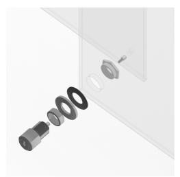
Install the keyed Lock assembly. Do not over-tighten the step nut. Check pin alignment to 6 mm hole by locking and unlocking (when in closed position).
