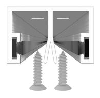
Fix the head guide to the top of opening. It's recommended to use two screws on each end and in the center (4mm diameter pre-drill required) predrill. Slide the door seal into each side as shown.
