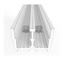
Fix the double track to the bottom of opening. It's recommended to use two screws on each end and in the center (4mm diameter pre-drill required).
