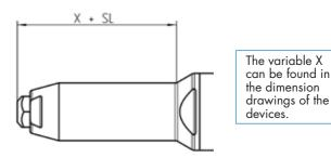
**Dimension X** = Standard steel head sleeve length (with standard nosepiece)
