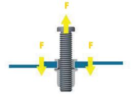
The thread must still turn smoothly in order to pass the test. Then the blind rivet nut is loaded again up to the overtorque.
