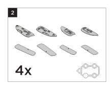
Use the icon on the footpads (5-8) to help identify the appropriate position on the vehicle and match anti-abrasion tape (12-15) to footpad (5-8).
