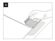
Use the clip tool (1) to carefully retract the rubber gasket at the arrow location.
