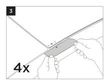
Apply anti-abrasion tape (12) to the front driver side of the vehicle by aligning the arrow on the glass with the arrow on anti-abrasion tape (12), and aligning the edge of the tape with the edge of the trim line.
