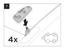
Place the front driver side pad (5) over the clip on the front driver side. Use the icon to help identify and install the correct pad (5-8) in the proper location.
