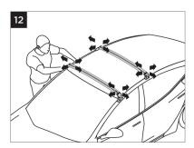
Test that the front and rear crossbars are securely installed by pulling vigorously in all directions.
