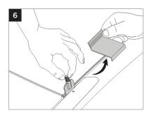
Remove the clip tool (1), being sure the clip (11) is engaged in the metal receiver under the glass. Pull up and wiggle the hook to be sure it's properly engaged. Be sure the center of the hook aligns with the arrow.
