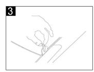
Carefully insert a clip at the arrow location. Make sure the clip is engaged in the metal receiver under the glass. Repeat this to install a clip on the other three corners of the car.
