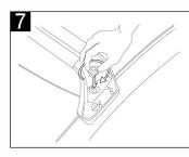
Install the nuts and tighten with spanner onto each of the towers. We recommend tightening to 2.5-3.5 Nm. To confirm the tower is properly installed, pull in all directions and ensure there's no movement.
