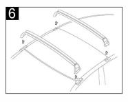
Ensure all four clips are engaged, properly aligned and in the upright position. Then, carefully place the front and rear crossbars over the pads.
