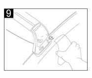
Install covers. Start with the bottom edge then press the top into place.
