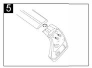
Place the front driver side pad over the clip on the front driver side. Use the icon to help identify and install the correct pad in the proper location.
