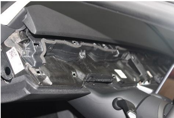
Picture 32 shows what the dashboard looks like after the cover removal.
