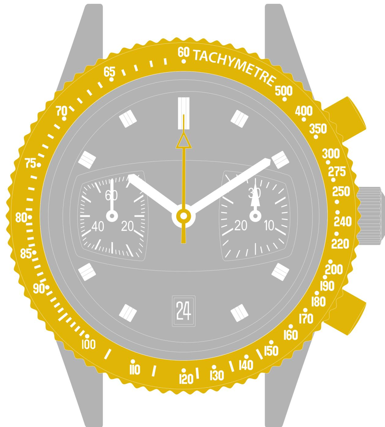
The bezel on your watch has a tachymeter function used to measure a speed or a flow rate using the chronograph function. Select the desired unit of measurement (metre, kilometre, mile, litre, etc.), activate the chronograph and stop it when the desired unit is reached. The centre seconds hand indicates the number of units per hour on the tachymeter scale.
