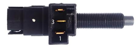
If you install the brake switch where the button is out then pushed in when applying the brakes, install the module red wire to terminal 1, brake light power out to terminal 2. If you install the brake switch where the button is normally in, but then pops out when brakes are applied, install module red wire to terminal 2, brake light power out to terminal 1. 12 volt + switched power to terminals labeled 3.
