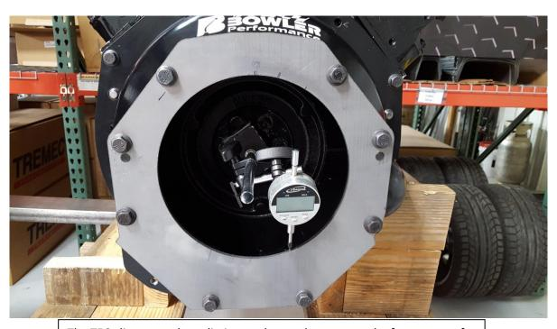
The T56 alignment plate eliminates the need to remove the front cover of the transmission. The procedure for dial indicating the alignment plate is exactly the same of any 4/5 speed bellhousing.
