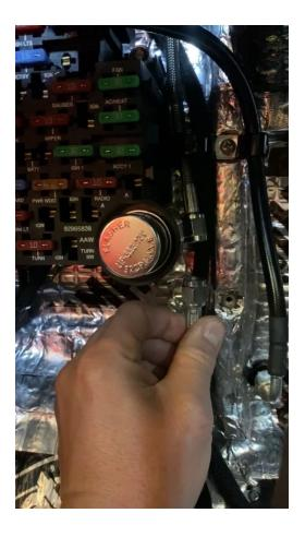
There are two hoses that make up the pressure circuit inside the truck. There is a 6" hose, then the adapter fitting for the pressure switch, and a 10" hose that attaches to the bulkhead in the floor. We have included and pre-installed a pressure switch into the clutch feed fitting. This is a safety part and should be wired into the starter relay. On the coil side of the starter relay use this switch to provide the ground. This will only allow the starter to engage when the clutch is depressed.
