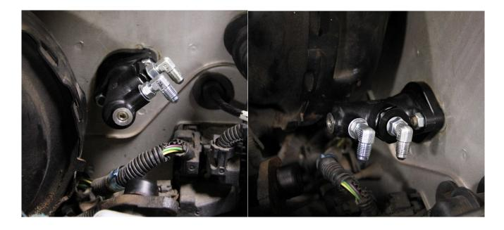
Step 9 - Once the new master cylinder has been secured to the firewall, go back un- der the dash and slip the rod end onto the clutch pedal pin. The plastic clip should secure it by snapping into place. At this point it will be easiest to check and make sure the push rod length adjustment is set correctly.
