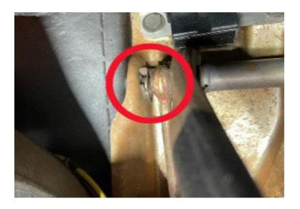
Step 3 - Use a 1/2" wrench to remove the 2 nuts that secure the master cylinder to the firewall and gently pull the master cylinder assembly out from the firewall and set aside.
