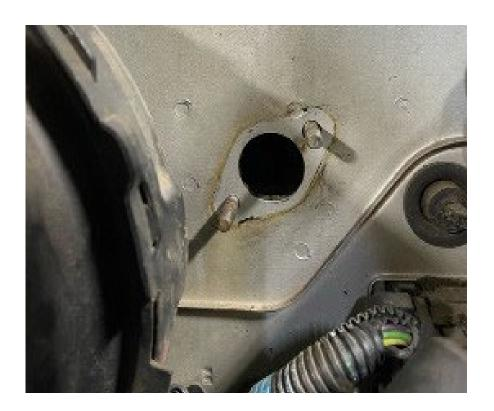
Step 7 - Slip the black anodized aluminum master cylinder spacer over the top of the studs.
