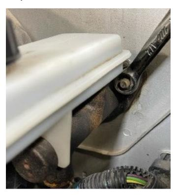
Step 4 - With the old master cylinder removed, assemble the new master cylinder assembly and ready it for installation. The new push rod uses a right and left hand threaded adjuster. For most trucks setting the distance from the center of the rod end to the master cylinder flange at 7 3/4" will achieve the correct pedal travel, but some adjustment may be necessary for your application.
