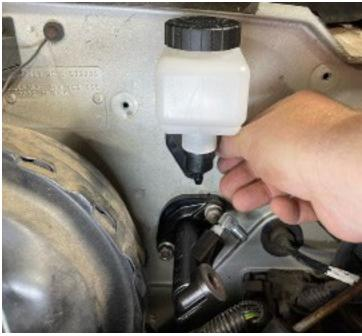
Once you have the reservoir mounted and the line connected from the reservoir to the master cylinder and also the line from the master cylinder to the bearing you are ready to fill with DOT 3 brake fluid and bleed the system. Please refer to the instructions that came with your release bearing for the proper bleeding procedure.
