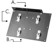
This background roller system has the motors pop-riveted into the tubes and it has mounting support plates at each end. The attachment brackets for these plates are shipped for ceiling mounting (A) but can be moved for attaching to the wall (D).
