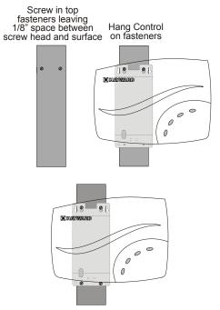
Screw in bottom fasteners securely.
