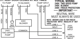
For single speed pump and/or 120 Volt equipment, follow wiring above except: 240 V. Single Speed Pump - Connect <u>both</u> BLUE and GRAY leads to LOAD 1 of pump.
