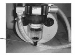
**MONTHLY:** The Part No. VTS529-1 filter element must be replaced once a month for proper vacuum and pump operation. Three (3) replacement filters have been included with your machine.
