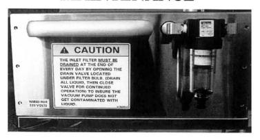
**DAILY:** Drain all moisture from the filter enclosure. Turn the drain knob counter clockwise to drain.
