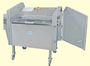
Md. 109PCM – right door open showing location of the thickness control gauge
