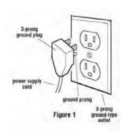
For your personal safety, this appliance must be grounded. This appliance is equipped with a power supply cord having 3-prong ground plug. To minimize possible shock hazard, the cord must be plugged into a mating 3-prong ground-type outlet grounded in accordance with local codes and ordinances. See Figure 1. If a grounded outlet is not available, it is the personal responsibility and obligation of the customer to have a properly grounded 3-prong outlet, installed by a qualified electrician.
