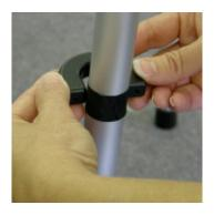
Select appropriate clamp for the tube diameter and place it around the tube in location cane or reacher holder is to be mounted.
