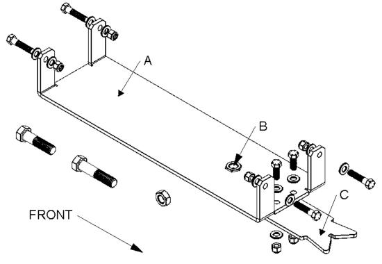
Position bracket (A) onto frame. Leave ½" of clearance between the top side of the bracket (A) and the bottom side of the wheelchair. The welded nut (B) should be positioned closer to the front, between the front wheels.
