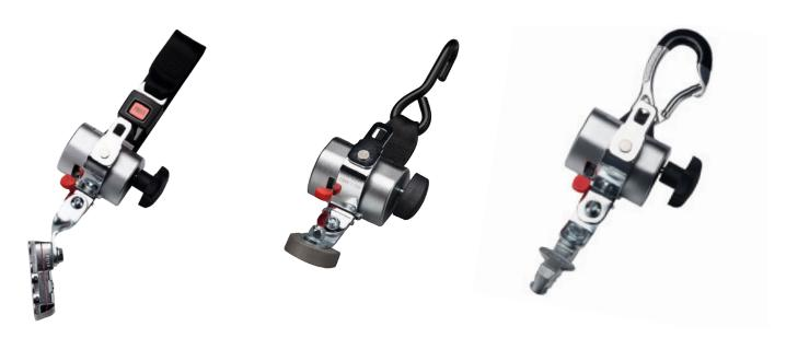
The ISO 10542 tested **SILVER**SERIES has a fully automatic pull-out and self-tensioning system. Its robust zinc diecasting cover is suitable for daily use in your vehicle. Various floor anchorage points with 4 stud fitting and mono fitting. Retractor system includes 4 retractor belts (or 2 retractor belts + 2 static belts) and one pelvis belt.
