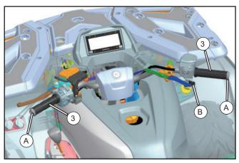
Stick the glue (6) to inside of the grip and the handlebar tube, then install the B type heat grip (3) and tighten the screw (A). Finally stick the thumb heater (B) to the throttle button.
