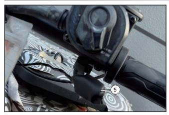
Put the heat shrink tube (5) on the throttle button, use a lighter to heat-shrink it.
