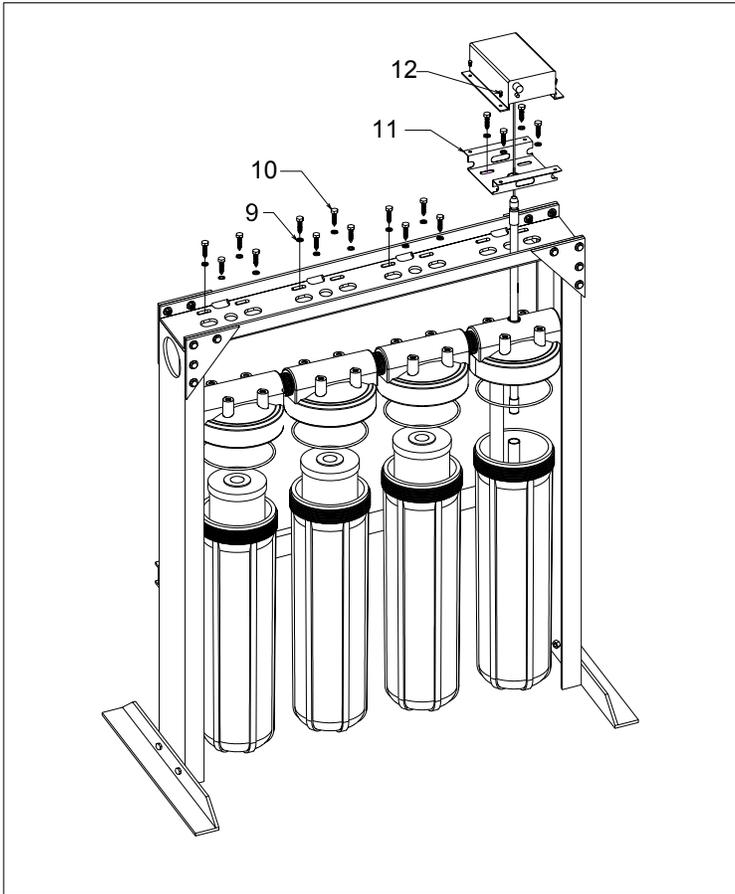
**Figure 5:** Module Attachment Points
