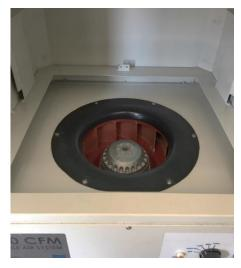
4. With the back panel off, open and install the HEPA filter with the gasket side facing down and place it directly on top of blower motor completely covering the opening to limit air-flow bypass.
