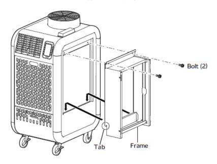
4. Insert the four (4) brackets of the plenum into the slots of the frame and secure the plenum to the frame with the four (4) bolts, which were removed in step 1 on page 3.
