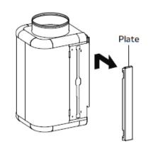
6. Insert the filter panel into the plenum as shown.
