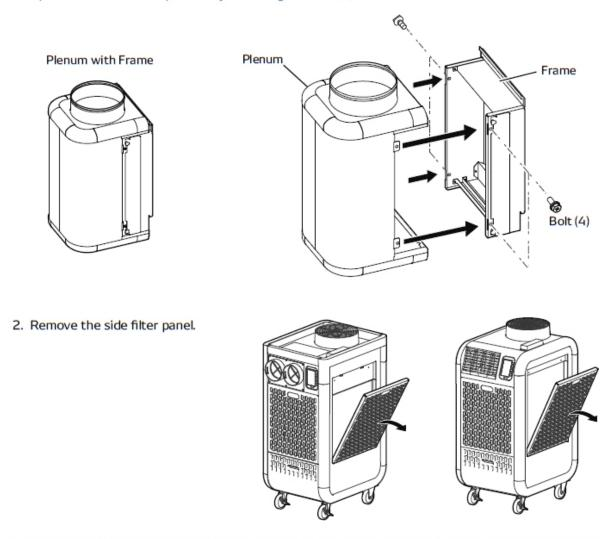
3. Attach the frame to the side of the unit by placing the tabs to the edge of the lower opening and secure the frame with the two (2) bolts supplied with the plenum.
