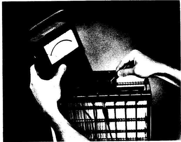
USE AN OHMMETER TO CHECK THE ELECTRONIC CELLS FOR SHORT CIRCUITS
