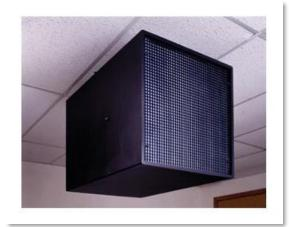
Air Cleaner be installed in areas that have 12-foot ceiling heights or more. The Mark 20 is equipped with 4 eye bolts installed 16" on center on top of each system for easy installation. The installation hardware also includes: 4 "S" hooks, 4 eye lags and industrial hanging wire. One (1) MARK-20 unit is recommended for every 10,000 cu. ft.
