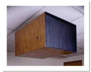
recommended that the Mark 15 Air Cleaner be installed in areas that have 10 - 12 foot ceiling heights. The Mark 15 is equipped with 4 eye bolts installed 16" on center on top of each system for easy installation. The installation hardware also includes: 4 "S" hooks, 4 eye lags and industrial hanging wire. One (1) MARK-15 unit is recommended for every 8,000 cu. ft.
