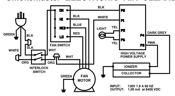
FIGURE 6 - 120V SCHEMATIC
