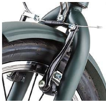
Typical Rim Brake (V-Brake)
