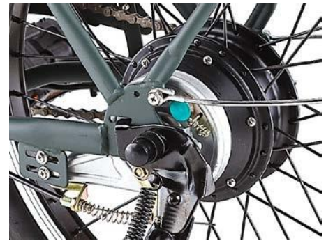
Typical Drum Brake
