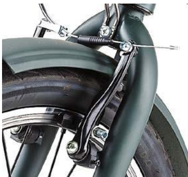
Typical Rim Brake (V-Brake)
