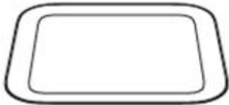
Crumb Tray This tray catches crumbs or small pieces that may fall to the bottom while loading or removing trays
