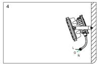
4. Connect the AC cable, Black cable joins to Live wire, white cable joins to Null wire, green cable joins to grounding.
