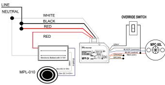
. When lights are manually turned off, switch must be returned back to the on position for the occupancy function as set.
