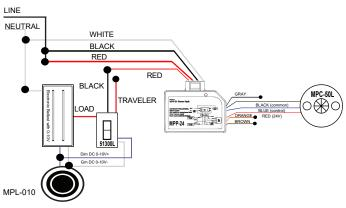
1. Daylight harvesting sensor supersede dimmer during daylight
