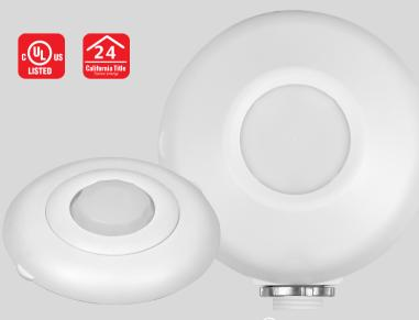
The MPC-50HD is a commercial grade line voltage high bay ceiling sensor that operates dimmable lights using passive infrared (PIR) technology. This unit is specifically designed for high bay and fixture mounted applications and it features interchangeable 360° fresnel lenses that provide up to 1200-2800 sq.ft of coverage area for ceiling heights from 8-50ft.
