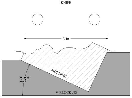
Due to a depth of cut greater than <sup>3</sup>/<sub>4</sub>" this knife will need to be used in conjuction with a customer supplied V-block, typically made of wood.
