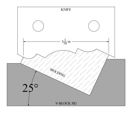
Due to a depth of cut greater than 3/4" this knife will need to be used in conjuction with a customer supplied V-block, typically made of wood.
