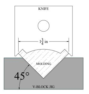
Due to a depth of cut greater than 3/4" this knife will need to be used in conjuction with a customer supplied V-block, typically made of wood.
