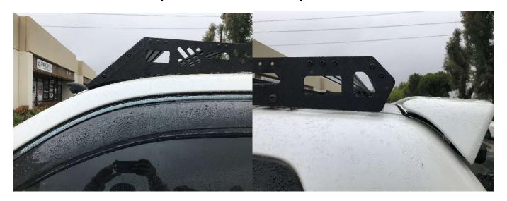
Once satisfied with placement tighten the sides 3/8 Mounting bolts.
