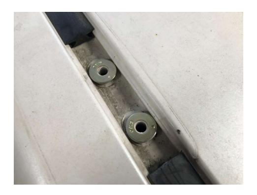
Add silicone inside and around, then place the 1" Aluminum spacer.
