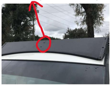
Then add the 2x elbows. With all the side bolts loose this will allow you to be able to insert the wind deflector in between the 2 side rails.
