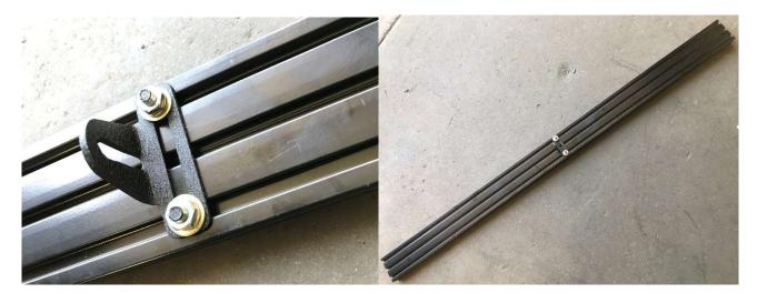
Carefully bolt up the first 3" rail with hangar brackets installed. Then space out the rest of the rails in the order above.
