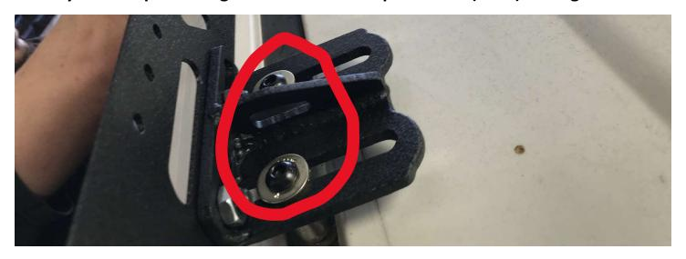
Final step is to bolt up the wind deflector bracket .
