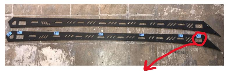
First Add the Deflector Hangar bracket to a 3" cross rail that will be mounted in the very front of the rack
