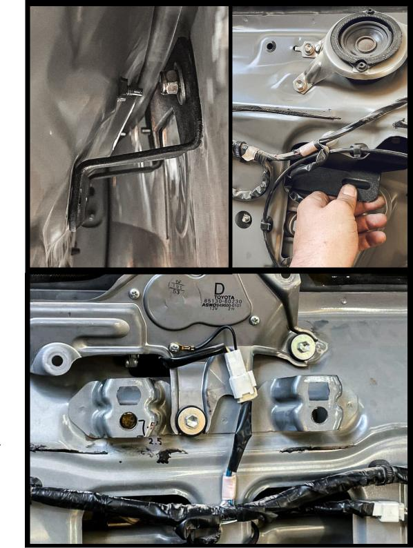
ONCE BOTTOM HOLES HAVE BEEN DRILLED YOU WILL NEED TO MOVE BACK TO THE INSIDE AND GRAB YOUR LOWER BACKING PLATE AND INSTALL IT IN PLACE.
