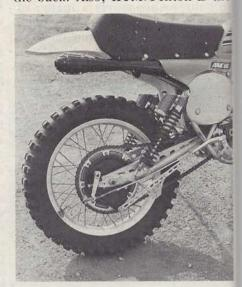
Marzocchi shocks have larger shafts and reservoirs. Chain guide moves up and down.
