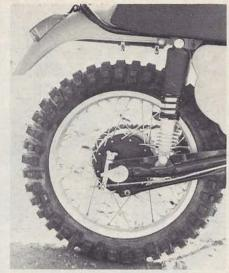
Semi-full-width-conical rear hub is aligned by two snail cam adjusters.
