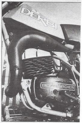
The rocketship chrome cylinder of Number One was so fast that it was too pipey to ride. The pipe is a modified YZ125E pipe.
