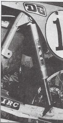
The rear suspension was handled by a short MX4 swingarm and Kayaba F-series air shocks. The shocks are a quick and clean fix.
