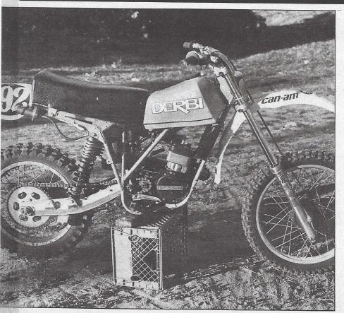
In its final form the latest Derbimobile featured Ohlins shocks, Thor swingarm, M. Robert rear fender and a Chrysler heater core.
