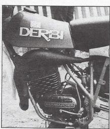
Number Three's engine was fired by a faulty non-stock Motoplat. For engines
