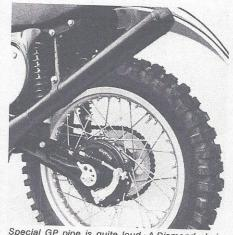
Special GP pipe is quite loud. A Diamond chain (% x %) rotates on a lightweight alloy sprocket.
