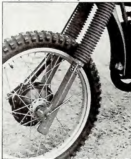
Forks are the 9½-inch Marzocchis, and are air adjustable. A cross-over tube keeps the pressure balanced.
