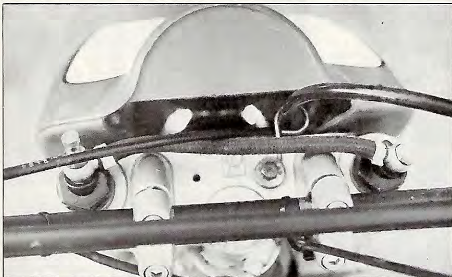
Once the forks loosened up, we used four to six pounds of pressure in the front end. The valve should be moved to the other side if the optional speedo is used—it interferes with the reset knob.
