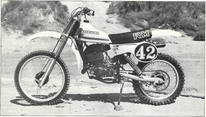
Cosmetically, the RM100T is cleaner than the N, with new fenders, seat and stickers. Reworked, internally, are the pipe, crank and timing. Suspension travel, seat height and ground clearance all took a slight climb this year.
